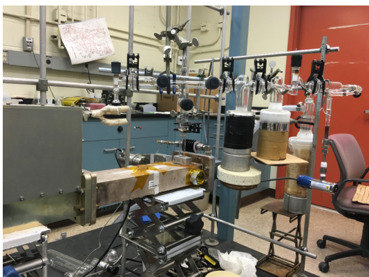
Fig. 1. Microwave/Condensation Apparatus
